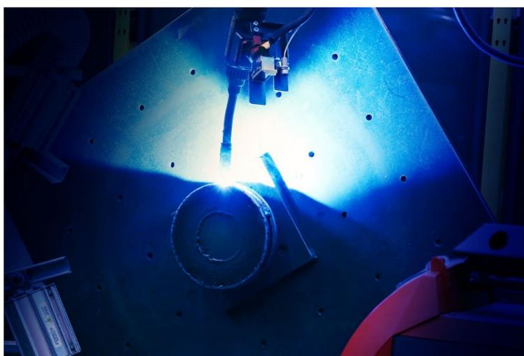
Figure 1 – Example of an industrial part being printed using WAM<sup>®</sup>
