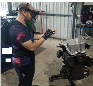
Caption: Technician utilising the industry specific Augmented reality headset to inspect the welding on an automotive oil sump
