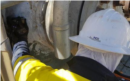
Caption: Advanced NDT Technician scanning a pressure vessel using Phased Array Ultrasonics
