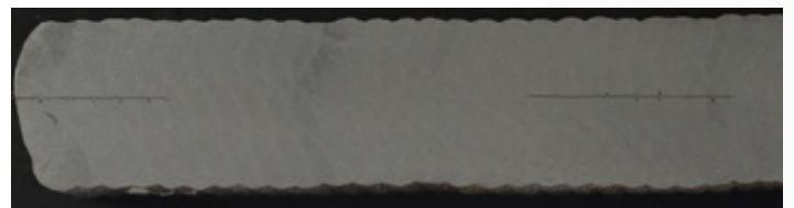
ER80S-B2 showing top and mid thickness hardness survey locations.
