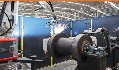
Designed for increased productivity, ARCEMY® Enterprise Edition is perfect for the facility that has medium to high manufacturing volumes but is a little tight on floor space. For the creation of larger parts, ARCEMY® Enterprise Edition introduces a 2.5 m robot reach combined with a 750 kg positioner.
